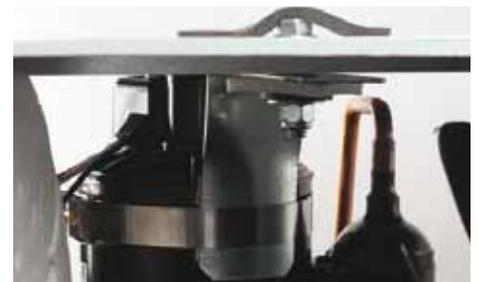
Compressor is bracketed at top and bottom to minimize vibration and movement
