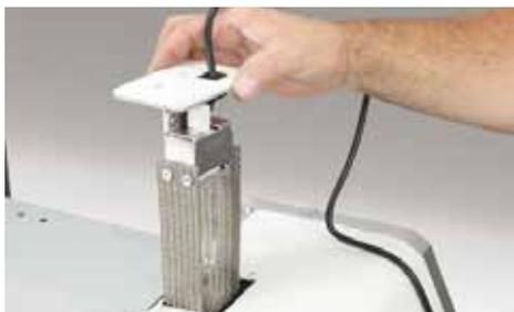
The integrated Breathe Easy™ air purifier is easily removed for UV bulb replacement
