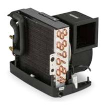
The TurboVap Series of direct expansion (DX) split-gas evaporators for boats is based on the revolutionary engineering advancements of the award-winning Turbo self-contained air conditioning system. Featuring a rust-free molded composite drain pan, condensate water is rapidly removed at one of two easy-to-plumb drain locations. The pan also has innovatively designed anti-slosh ridges and "positive flow" channels to ensure condensate does not spill even in the roughest seas.
