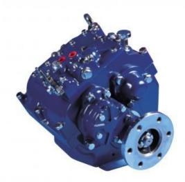
The hydraulic operating system functions on normal lubricating oil of the same viscosity as that used in the engine, avoiding the need to use automatic transmission fluid, and ensures rapid response to movements of the operating lever for good boat handling. The operating lever has a positive neutral detent and is suitable for use with proprietary single lever remote control operating systems.
