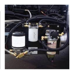
700 Series fuel filter/water separators come equipped with a state-of-the-art fuel priming pump for easy priming. The 12 vdc roller-cell fuel pump offers the benefits of an electric ondemand priming pump at a push of a button, and the 24 vdc brushless version directly drives the gerotor creating a unique, positive on-demand displacement pump.
